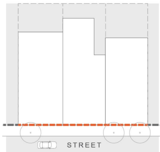
Figure 13 Buildings with ground floor retail should generally be built to the front boundary to create a consistent active street wall.
