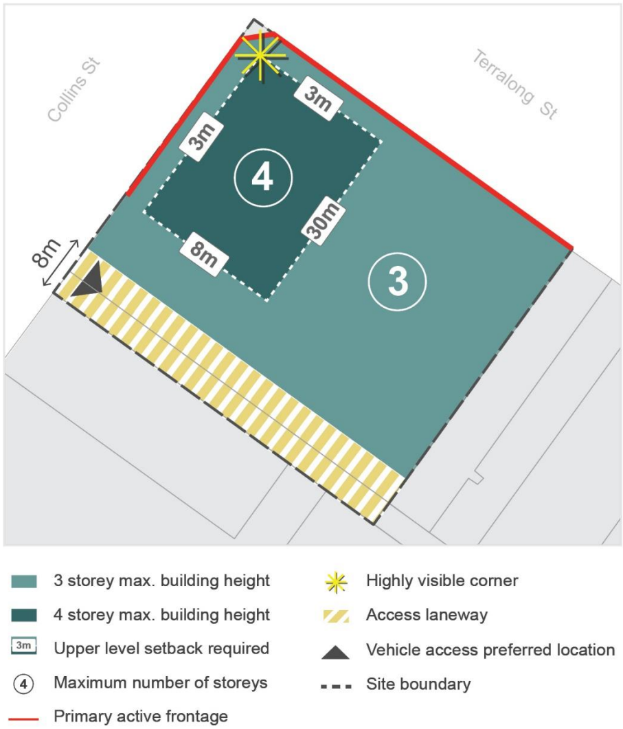
Figure 41 Sample Corner Site development control plan located at 106 Terralong Street. Other corner sites may vary – refer Figure 15 - Figure 18.
